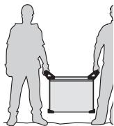
Never lift the machine while there is a gas cylinder on the support shelf. A clear path is available when moving the item. The removal of the wire reel from the machine is recommended before undertaking any lifting operation.
