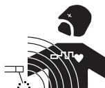
The electric currents flowing through a conductor cause electrical and magnetic fields (EMF). The welding current generates an EMF field around the welding circuit and the welding equipment.
